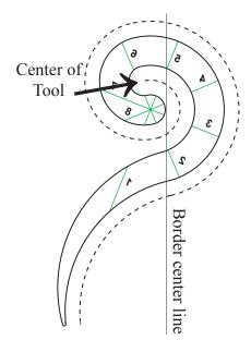
1. Place the Nautilus Baby Long Tail Tool on the lengthwise center marking of the border, as shown above. Anchor the stitching line and stitch around outside edge of the tool to center of the tool.
