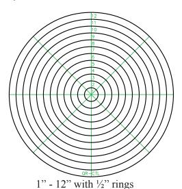
This template increases size by 1" with each ring. 1/8" thick: Part # QR-CT4 1/4" thick: Part # QR-CT5
