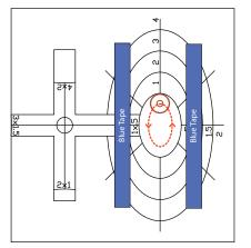
Pick an oval size. Remove key from template in order to position foot on the inside of the Nested Mini Ovals. Replace key being sure to match key to oval desired. If you use one of the smaller sizes, you might find it useful to use blue painter's tape to help hold the pieces when moving the template. Stitch a complete oval. Needle down.
