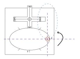
Rotate the template to the horizontal crosshair as shown above.
