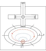
Remove second ring. Turn key to match new oval size. Slide template to foot position. Stitch a complete oval.
