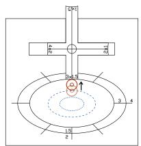
Remove second ring. Turn key to match new oval size. Move foot to edge of new oval.
