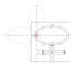
Rotate the template to the horizontal crosshairs as shown above and stitch a complete oval.
