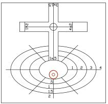
Remove key from template in order to position foot on the inside of the Nested Mini Ovals. Replace key being sure to match key to oval desired. Position foot at the bottom of the oval.
