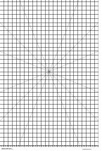
Whole Cloth Grid Overall Size - 25" x 38" Grid Size - 24" x 36" Measurement - 1" grid with 1/8" increments on side Guide Line: 22<sup>1</sup>/<sub>2</sub>°, 45°, & 90°
