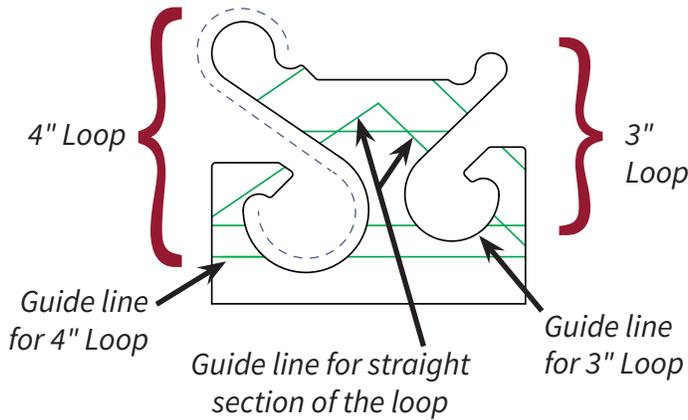
MQT-LTL is ¼" thick. HMQT-LTL is ⅜" thick.
