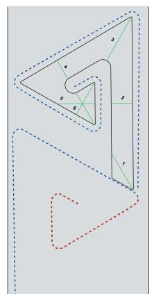
4. Move the Nautilus Delta Tool, flipping it so it is facing the opposite direction as before, with the longest edge again along the seam line and begin stitching around the tool until you reach the center.
